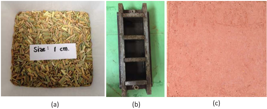
Figure 5. (a) Sample of rice straw fibers cut in 10-mm. size, (b) The ASTM standard size steel mold used to sample specimens for compression test, (c) a sample finished product in 300 mm. x 300 mm. x 10 mm. dimensions
